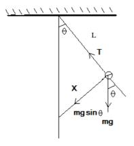
First of all we have to make a few assumptions which are needed for making the experiment to be successful. Those assumptions are: the string is weightless, the ball is completely spherical, and the angle between the string and the normal is too small so that q = sin(q) = tan(q) where q is the angle between the string and the normal measured with radian measure which is without a unit.
